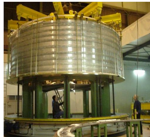
*Preparation of a module for VPI impregnation*
