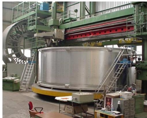
*Cylinder vertical milling machining*
